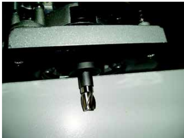
Fig.9. Properly protruding milling cutter.
