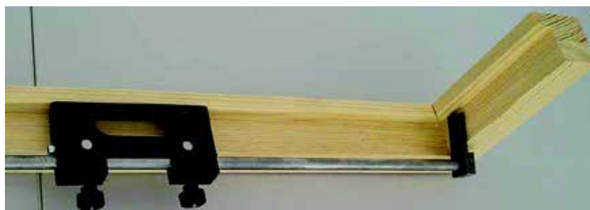
Fig.5. Proper arrangement of the end stop and rest buttons.
