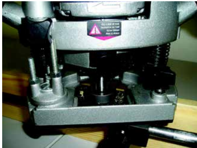
Fig.8. Milling holes 29x69,5x37 using three passes.
