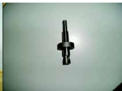
Fig.14. Arrangement of milling cutter.
