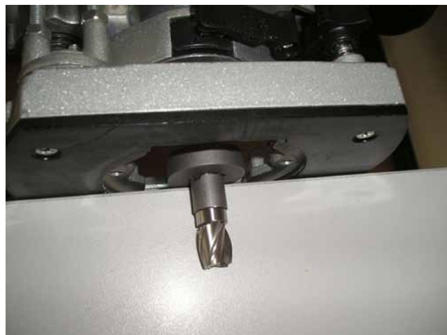
Fig. 9. Properly protruding milling cutter.
