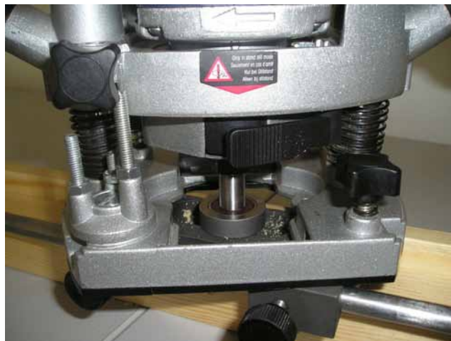
Fig.8. Milling holes 29x69,5x37 using three passes.
