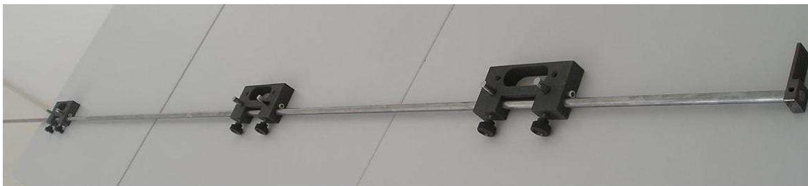
Fig.3. Master with frames on the slideways.
