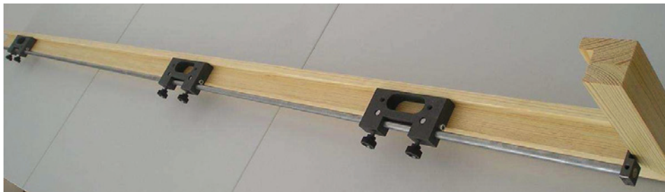
Fig.4. Slideway with frames on the door frame.
