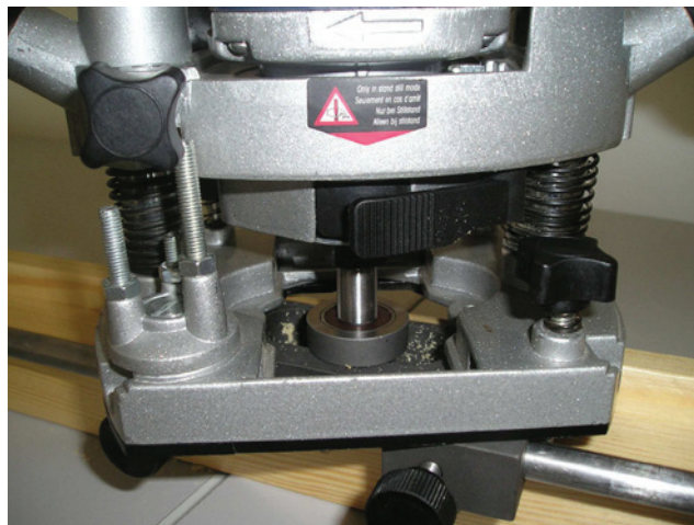
Fig.8. Milling holes 23x60x30 using three passes.
