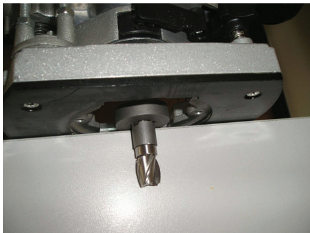
Fig. 9. Properly protruding milling cutter.
